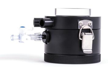
Temperature of the sample can be accuratley controlled by connecting an external circulating water bath (not included) to the water jacket inputs of the LD1/2
