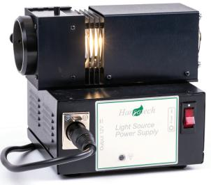
The lamp housing contains a cooling fan, infrared reducing "Hot-Mirror" and optics to provide light with minimum variation of intensity across the beam and little divergence from parallel. 2 slots are provided to accept 50mm square optical filters or a manual shutter plate.
